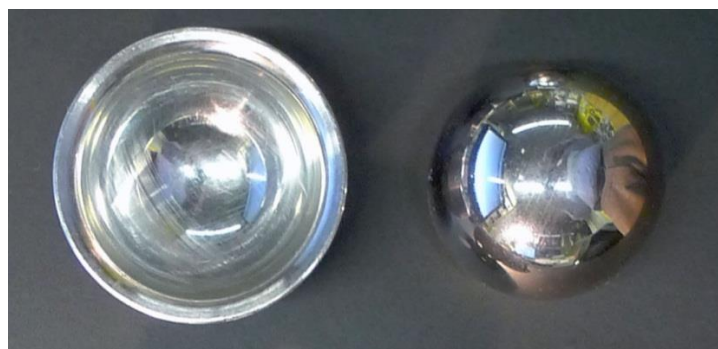
Figure 3: The two articulating components of contemporary Category 1b1 MoM bearing articulations with a diameter of 36mm. The CoCr-alloy metal cup liner has a thinner wall thickness as the 32mm diameter liner shown in Figure 2 and such fits in the same uncemented hip socket. (Source: M.Morlock)
